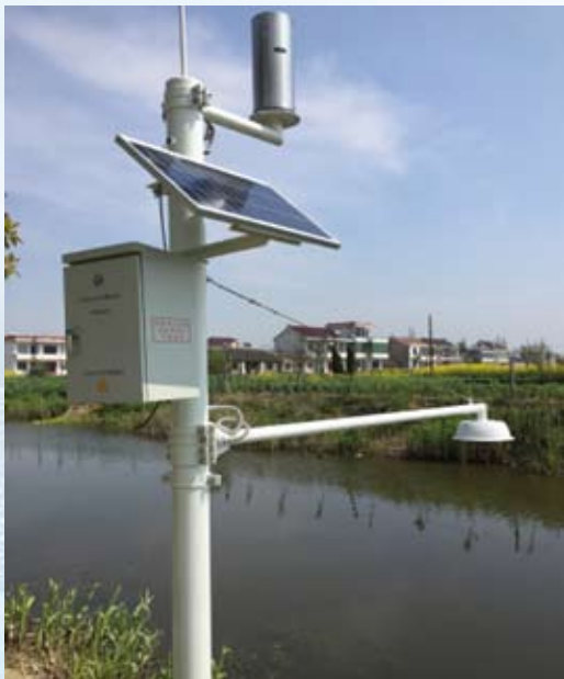
• 雷达水位计测站 Radar level meter measuring stations
